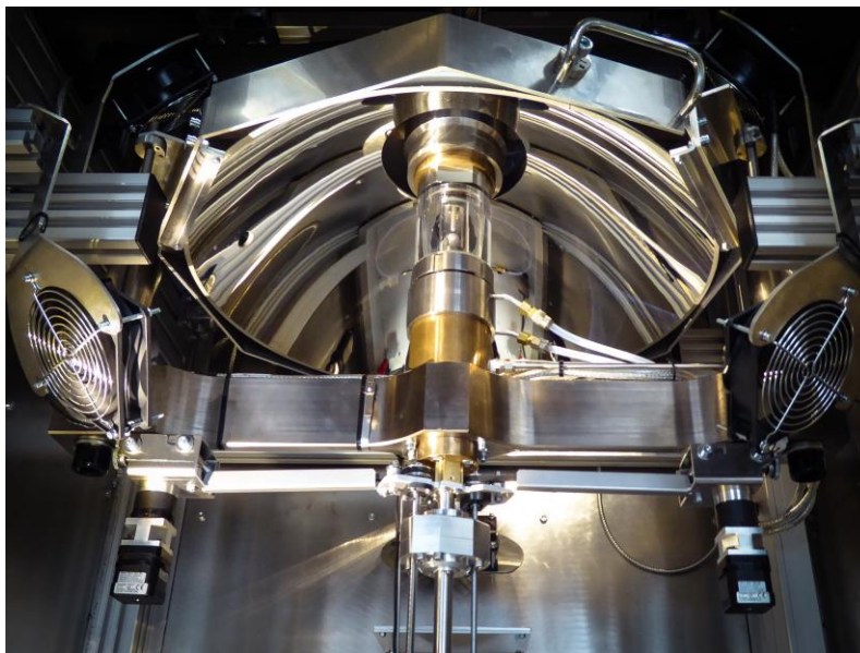
Picture 2: The process chamber is located at the focal point of the upper mirror of the HKZ. Here, the crystal growth takes place at temperatures of up to 3000 °C and a gas pressure of up to 300 bar.
